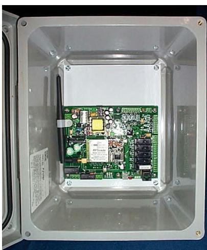
Typical examples show RFScada devices with license free ISM modules and internal antennas installed. On the left is the lower powered version, and the higher powered (SS1) version is on the right.
